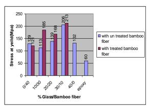
Fig.1. The variation of Stress at Yield with ratio of % Glass/Bamboo fibers Reinforced polyster composites
