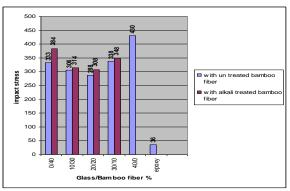
Fig. 3. The variation of impact strength with the ratio of % Glass/Bamboo fibers reinforced polyster composites
