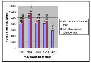
Fig. 2. The variation of Flexural modulus with ratio of % Glass/Bamboo fibers reinforced polyster composites
