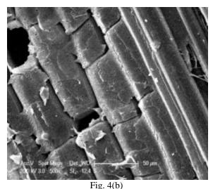
Fig. 4 (a) & (b) represents the fractograms of untreated bamboo fiber at two regions with a magnification of 100X.
